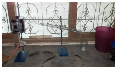
Figure 1. RAP Asphalt Distillation Extraction
